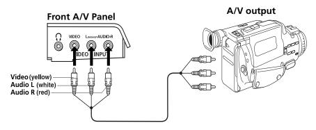
For model KV-13M42, this connection can be made to the Audio/Video input located on the rear of the TV.
